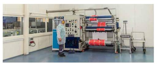
The production of unadulterated dairy packaging for children in contact with food takes place in a clean room equipped with high-efficiency particulate air (HEPA) filters. Clean room microbiological activity is regularly measured and recorded with devices from accredited laboratories, including air, packaging surface, and personnel hands.
